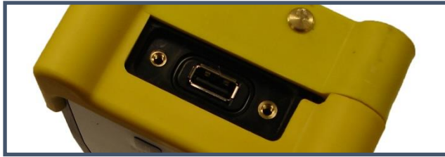
Handheld & Panel Mount - Remove the top cover on the controller with a phillips screwdriver.
